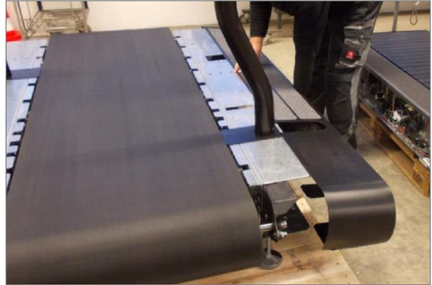
Fig. 58 Pro/Pro XL assembly, side covers
